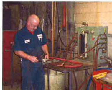
Water Check & Silver Plating Ends
