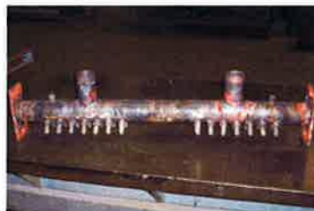
Dual Manifold After Brazing
